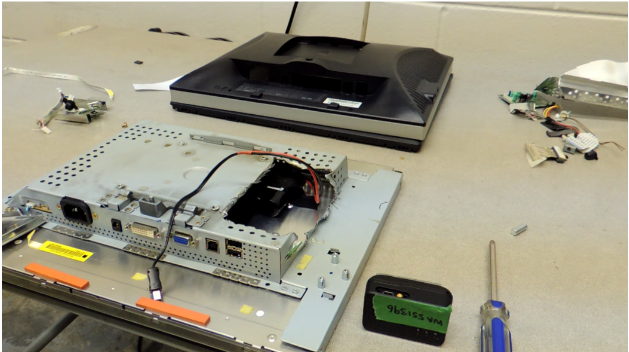
LCD with tracking device. Deployed at Interconnection facility in Seattle, WA on 1/29/16. Note numerous wires and parts have been cut, and large chunks of circuit board removed, making this completely non-functional and with an obvious tracker installed in the back.
