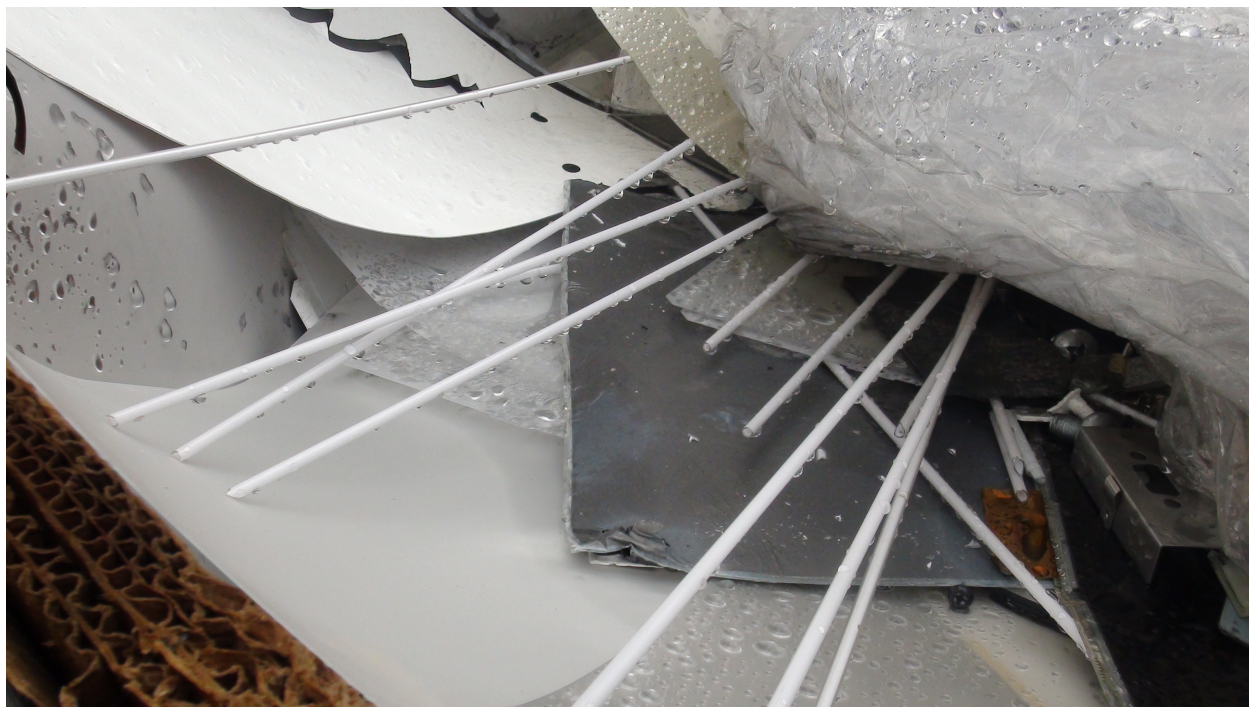
Broken CCFL tubes from LCD monitors near workstation where equipment was being dismantled by hand. Image from December 2015 BAN visit to Deep Bay Road location in New Territories, Hong Kong. Copyright BAN 2016.
