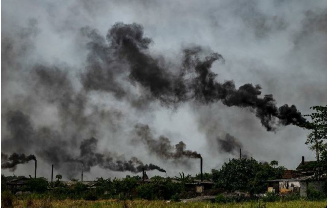
Figure 5. Nonrecyclable plastic scraps were used as fuel and openly burnt to cook soybean for making tofu, releasing dioxin to the air, producing toxic ashes and microplastics that will contaminate foodchain
